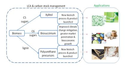
The lignin stream will be purified to enhance its value added application (e.g polymer building blocks, green chemicals, fibre) thus ensuring the complete utilisation of biomass.
