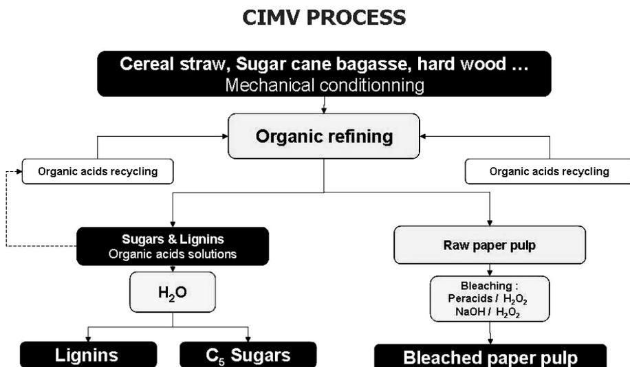
Figure 1. The CIMV process biorefinery.
