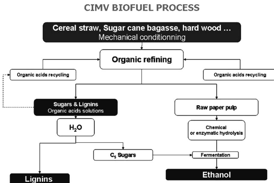
**Figure 4.** The CIMV bioethanol/lignins biorefinery.
