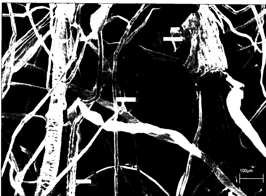
Fig. 1 SEM photomicrograph of a crude pulp sample obtained by rice straw cooking in organic acid media.
