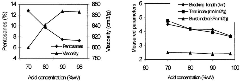
Fig. 2. Influence of acid concentration on pulp mechanical and chemical properties (cooking conditions: temperature, 100°C; time, 60 min).
