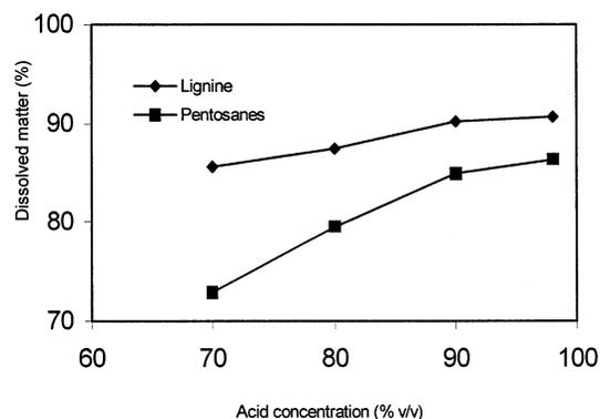
Fig. 1. Effect of formic acid concentration on dissolved matter concentration during rice straw cooking.
