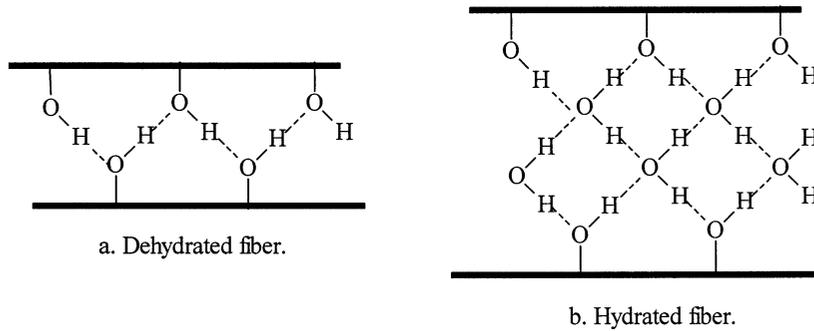
Fig. 3. Hydrogenous linkages between (a) dehydrated and (b) hydrated fibers (De Pascoal Neto, 1992).
